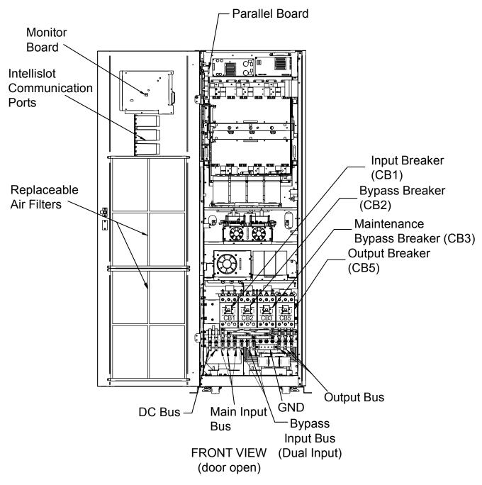
Figure 30 Liebert<sup>®</sup> NX<sup>™</sup> 40-120kVA main components—typical unit
